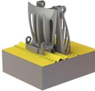
A unique feature of AM processes is the ability to build an assembly of parts. Crucible fully exploited this ability by building the sliding clamp that locks the belt in place as part of the main body, increasing strength and eliminating assembly time.
