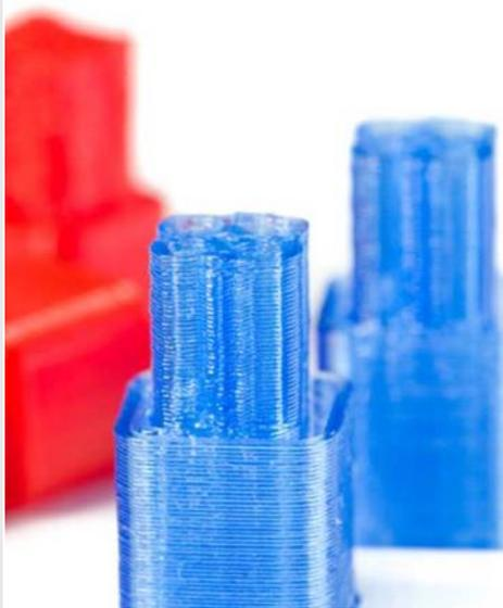
FDM parts showing layers prior to finishing
