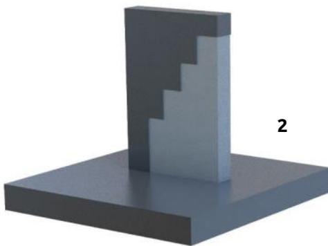
In image 2, however, the downward facing surfaces of the dark grey material needs supporting by the light grey material as it builds upwards, or the 'steps' would otherwise distort or collapse.
